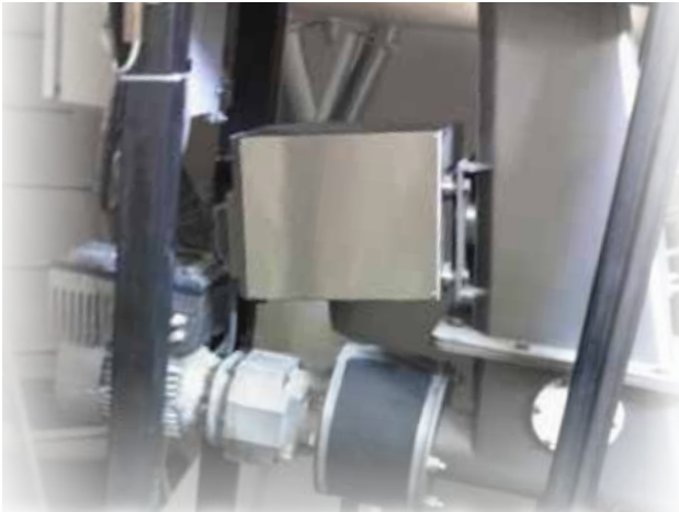
Wheat Flour Measurement of wheat flour using the optional Flour Measurement Chamber.
