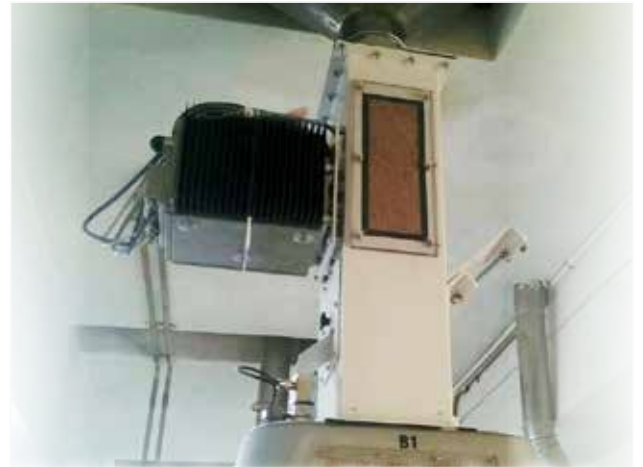
Whole Grain Measurement of wheat in a flour mill using the optional Whole Grains Measurement Chamber.
