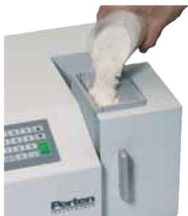
The Inframatic 9140 Flour Analyzer is a Near Infrared (NIR) spectrometer specifically designed for the analysis of flour. Its unique sample presentation system completely removes operator influence as a source of error making the Inframatic 9140 the most accurate flour analyzer available.
